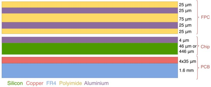
**Figure 4.9:** Simplified schematic cross section of the materials of one plane. The drawing is not to scale.
