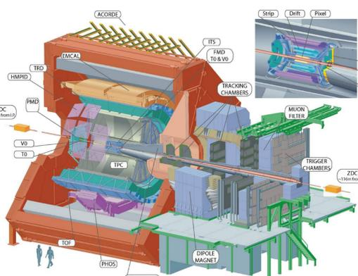
Fig.1 Schematic view of ALICE at the LHC.
