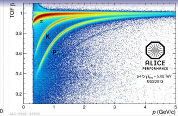
Fig.4 Velocity of particles as a function of  $p$  measured by the Time Of Flight detector (TOF).
