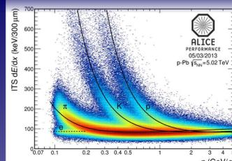
Fig.2 The specific energy loss as a function of momentum  $p$  in the Inner Tracking System (ITS).
