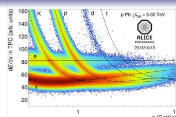
Fig.3 Specific energy loss  $dE/dx$  as a function of momentum  $p$  in the Time Projection Chamber (TPC).
