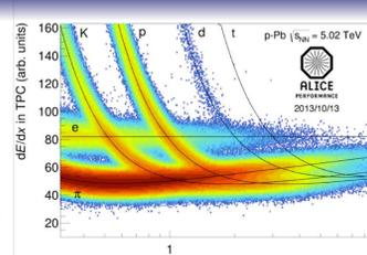
Fig.3 Specific energy loss  $dE/dx$  as a function of momentum  $p$  in the Time Projection Chamber (TPC).
