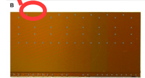
The cross-sectional image (A) and the photograph (B) of the ALPIDE chip
