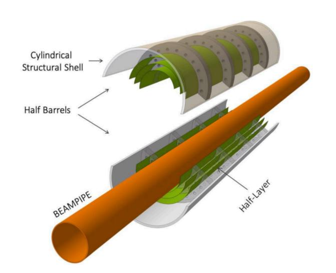
R=18, 24, 30 mm (beam pipe: 16 mm )
